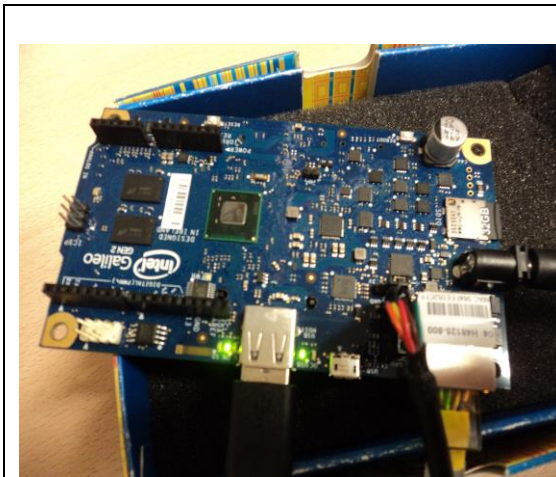
Figure 2. Galileo board using FTDI cable during cross compilation of Java OpenCV code on the board
