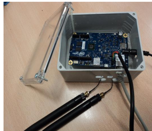
Figure 3. Galileo board with Wi-Fi shield configured
